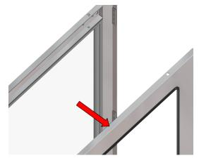
6. After removing door edge screws, detach the top door frame.
