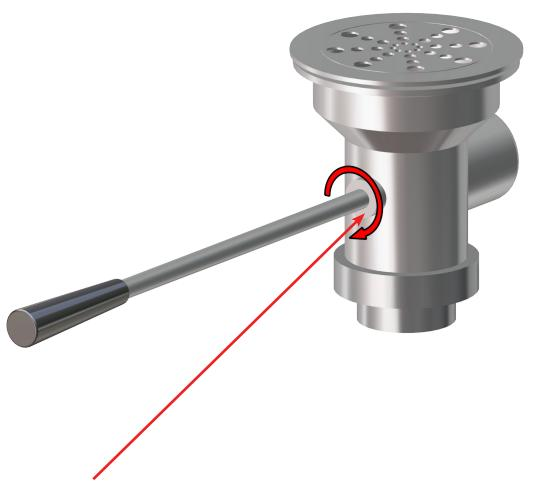
To adjust the handle on the Lever Handle Waste Drain (to prevent leaking), tighten the handle hex nut with a wrench.
