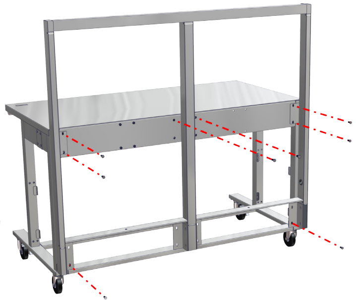
Fig. 1: Shipping position - remove bolts
