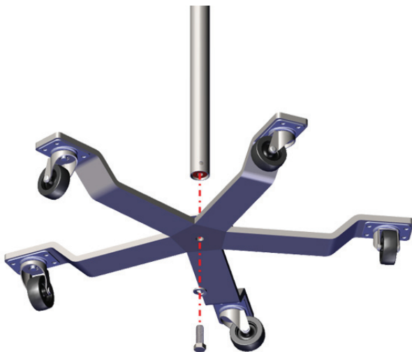
Fig. 4: Assemble Bolt, Washer, Base and Pole
