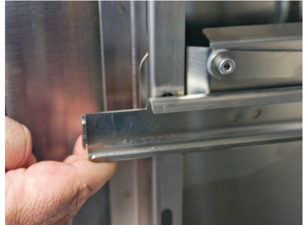
Fig. 11: Lift Rail up
