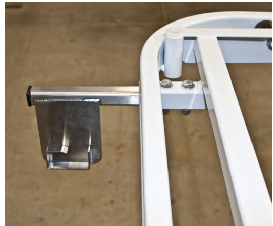
Fig. 8: Left side roll bracket assembly installed.
