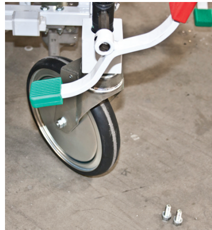
Fig. 5: Bolts removed and wheel unlocked
