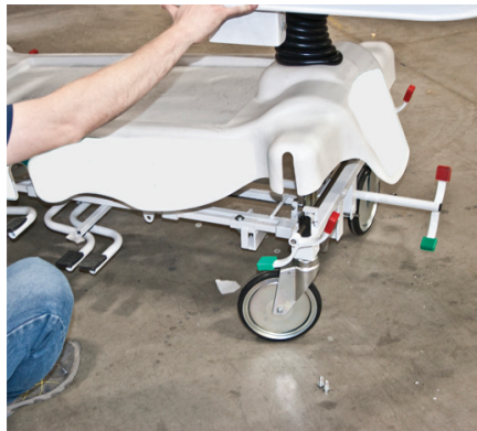
Fig. 6: Rotate wheel counter clockwise 360 degrees.
