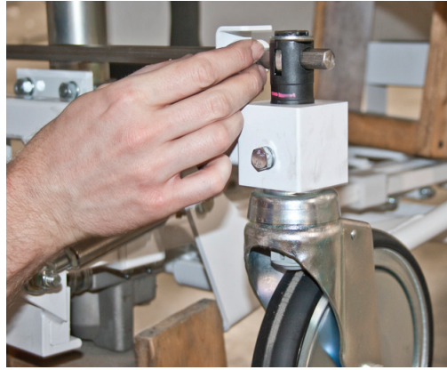
Fig. 13: Drive Hex Bar into replacement caster
