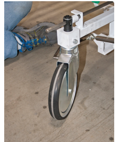
Fig. 5: Brake Pedal Removed
