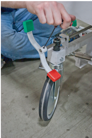
Fig. 3: Use Allen Wrench to loosen Brake Pedal.
