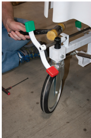
Fig. 4: Use rubber hammer to remove Brake Pedal
