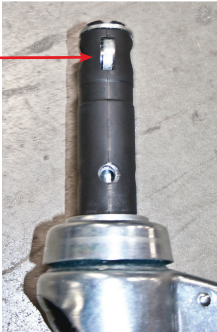
Fig. 14: Total Lock Gear Position
