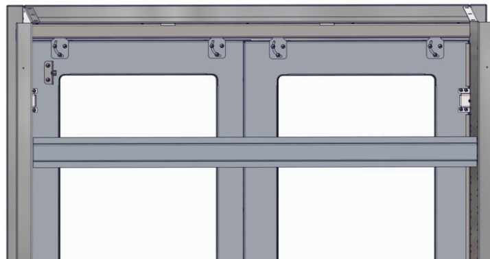
Fig. 3: Top inside of sliding doors
