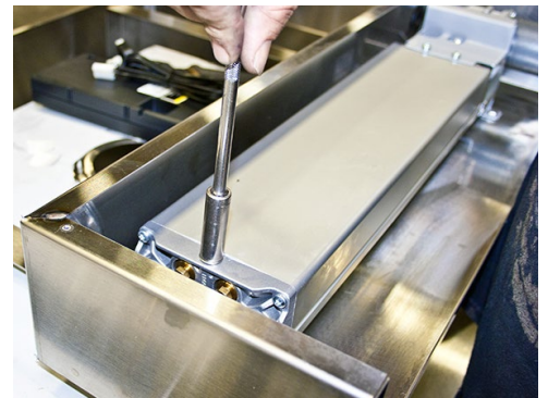
Fig. 32: Long bolt at pump head end
