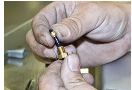
Fig. 26: Hydraulic screw & ferrule
