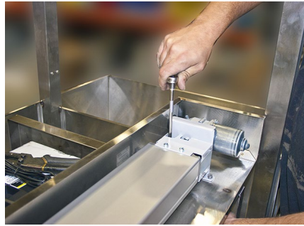
Fig. 15: 2 bolts at pump back end
