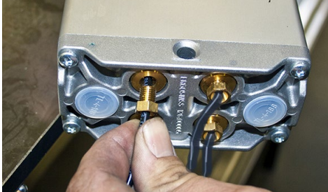
Fig. 27: Insert prepared line
