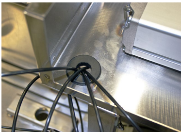
Fig. 24: Thread lines thru grommet
