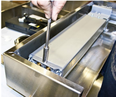
Fig. 14: Long bolt at pump head end
