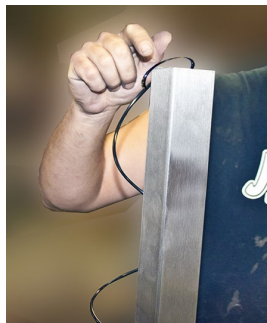
Fig. 18: Thread leg line
