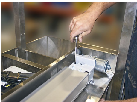
Fig. 33: 2 bolts at pump back end
