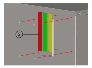
4. Line up all 4 holes and install screws into holes the put nuts on from the inside and tighten.
