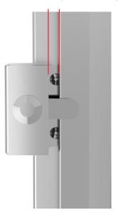
3- After locating lock box on the side of cabinet, drill and tap 10-32 holes for mounting screws. Use a screw with a star locking washer and locking hex nut on the inside. (Note: the side must be removed to attach the locking hex nut to the screw)
