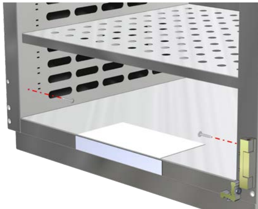
Fig. 30: Remove Interior Cabinet Screws - Glass Door Unit
