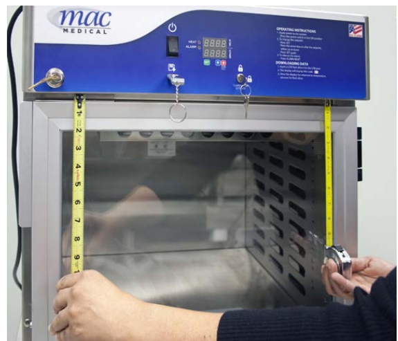
Fig. 68: Check Alignment - Square Door
