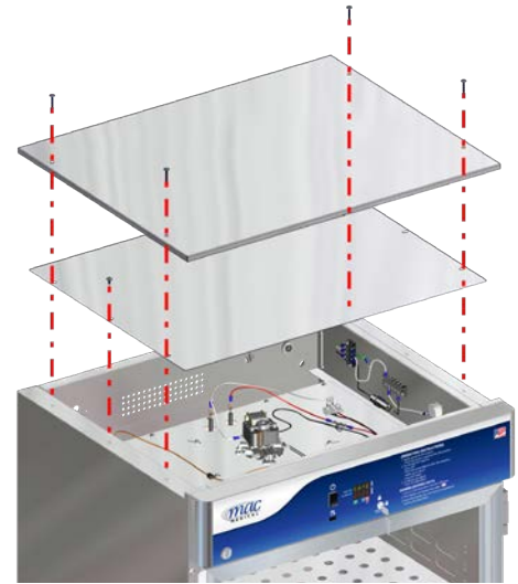
Fig. 29: Remove Top Panels
