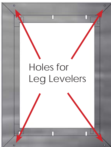
Fig. 8: Holes in Cabinet base
