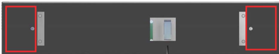
Fig. 34: Cut Out Rectangular Sections from Gasket
