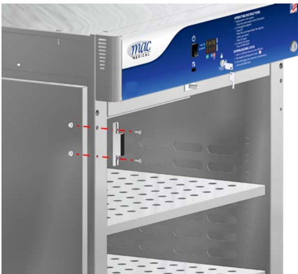
Fig. 55: Install Male Hinge Halves in New Position
