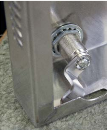
Fig. 41: Assembled Cam Lock
