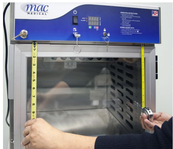
Fig. 68: Check Alignment - Square Door
