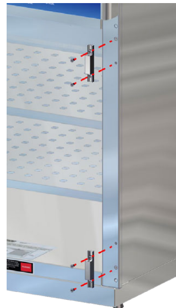
Fig. 46: Detach Glass Door Hinge - Male Half
