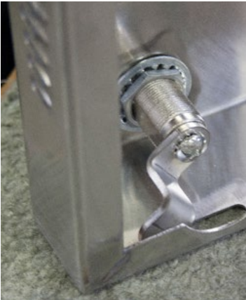
Fig. 41: Assembled Cam Lock
