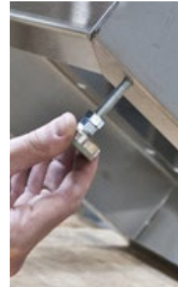
Fig. 9: Insert Leg Leveler into base
