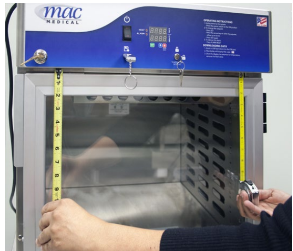
Fig. 68: Check Alignment - Square Door
