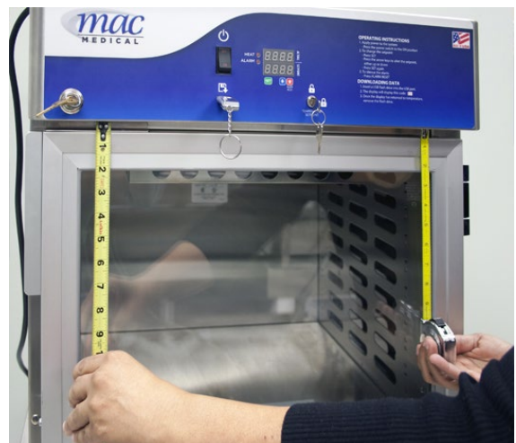
Fig. 68: Check Alignment - Square Door
