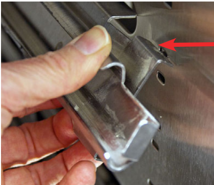
Fig. 20: Inserting Top Channel Tab
