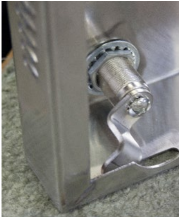
Fig. 41: Assembled Cam Lock
