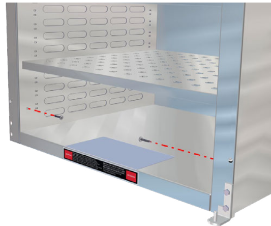
Fig. 31: Remove Interior Cabinet Screws - Steel Door Unit
