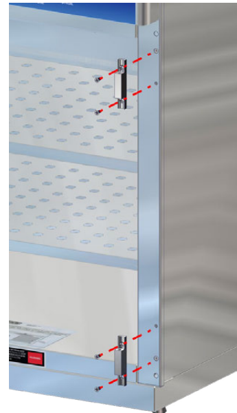
Fig. 46: Detach Glass Door Hinge - Male Half
