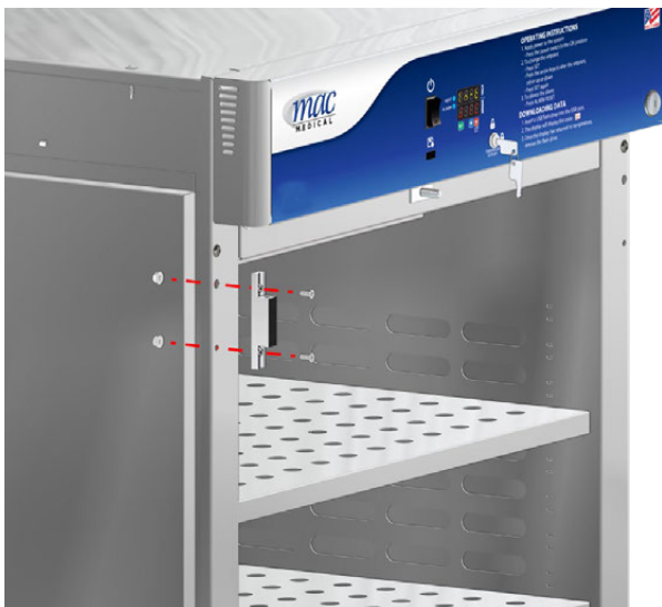
Fig. 55: Install Male Hinge Halves in New Position
