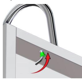
Fig. 9: Secure spout with bushing
