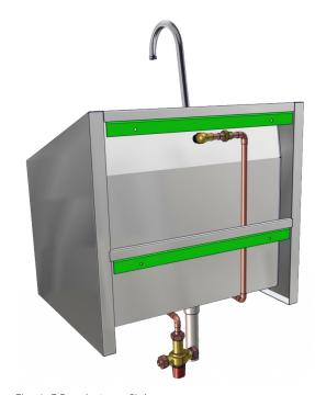
Fig. 6: Z Brackets on Sink
