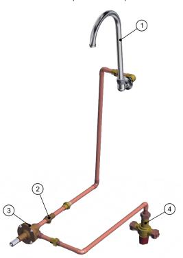
Fig. 14: Manual knee operated sink plumbing
