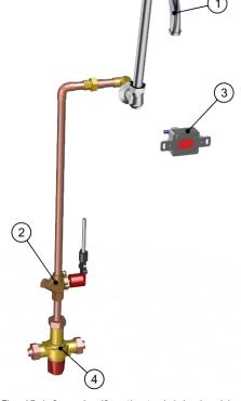
Fig. 15: Infrared self-activated sink plumbing
