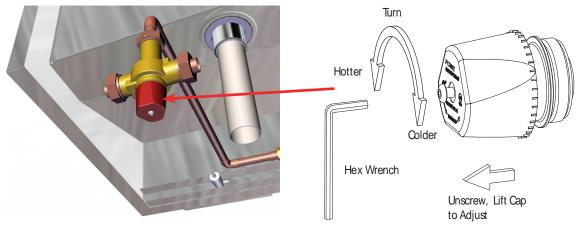
Fig. 12: View of Mixing Valve on sink
