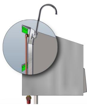
Fig. 5: Cross Section Showing Z Bracket Locations
