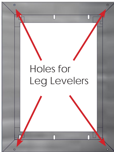
Fig. 7: Holes in Cabinet base
