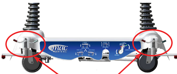
Brake/Steering Pedals (side view) in horizontal (non-depressed) position
