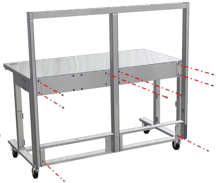
Fig. 7: Shipping position - remove bolts
