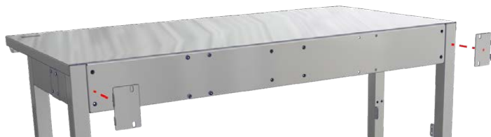
Fig. 8: Remove shipping brackets
