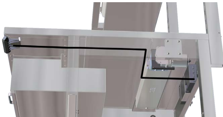
Fig. 26: Connect memory pad cord to power supply
