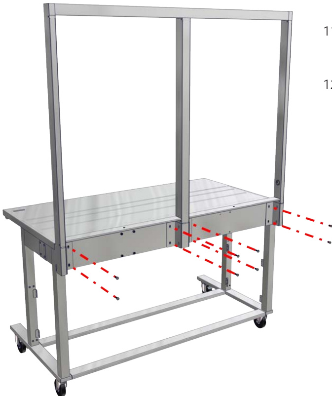
Fig. 9: Raise back bracket & insert bolts
