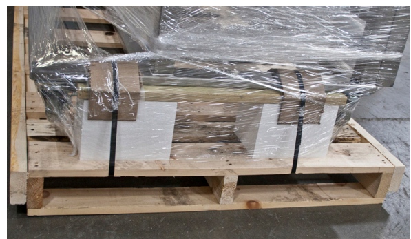
Fig. 6: Foam blocks protecting Casters
