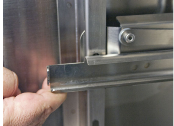
Fig. 11: Lift Rail Up
