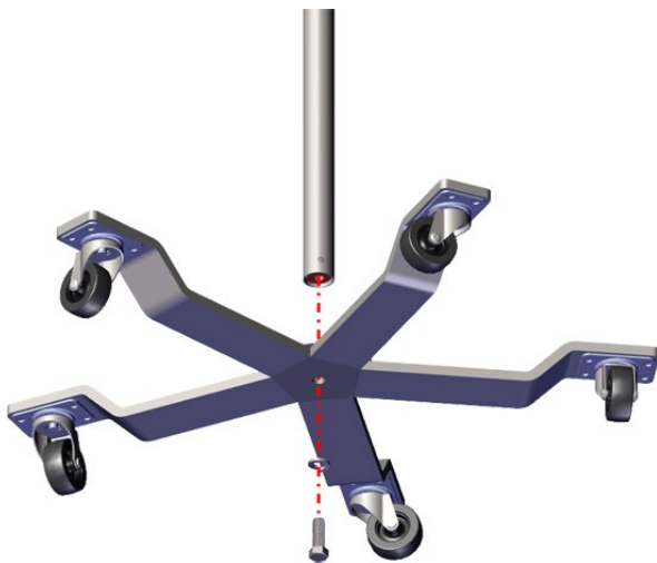
Fig. 4: Assemble Bolt, Washer, Base and Pole
