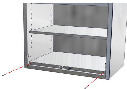
Fig. 4: Remove Front Screws
