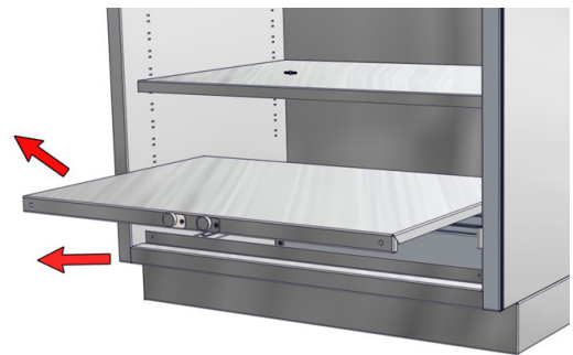
Fig. 12: Remove Cabinet Bottom
