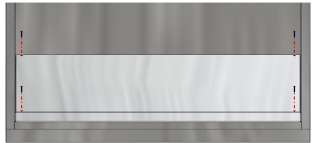
Fig. 16: Remove Four Top Screws
