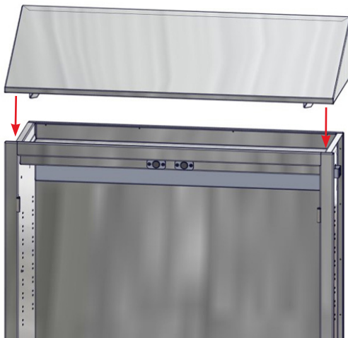
Fig. 2: Lower Sloped Top onto Cabinet
