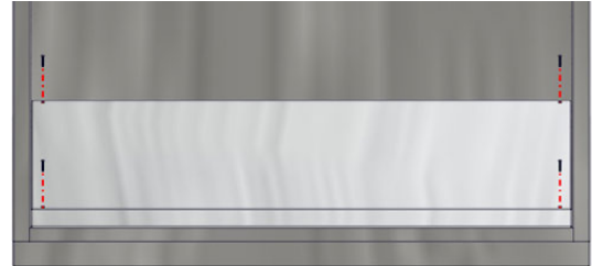
Fig. 15: Remove Four Top Screws
