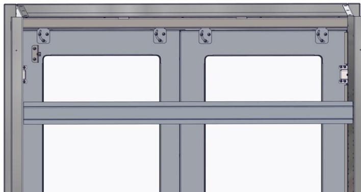
Fig. 23: Top Inside of Sliding Glass Doors
