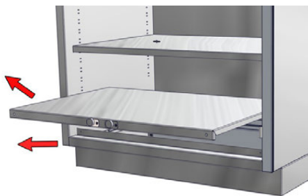
Fig. 13: Remove Bottom Panel
